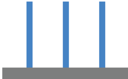
Wet etch pillar into SiO 2 wires
