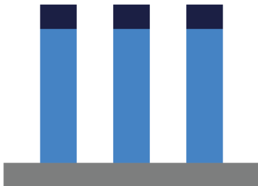
Stepper lithography and dry etch to form SiO 2 pillar
